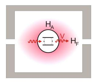
• Two-Level Atom  $H_A$ , • Photon-Field  $H_F$  • Interaction: V
